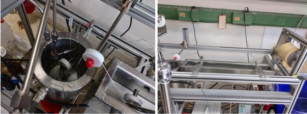
Extrusion of the photocatalytic fibers with the dry-wet phase inversion process in spinneret set up
