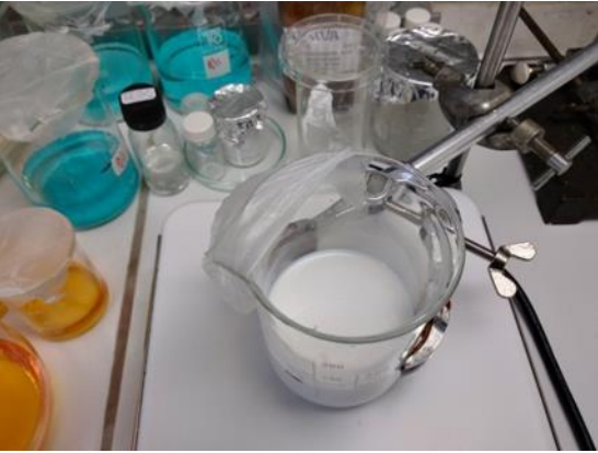
Preparation of the PVDF/TiO 2 solution
