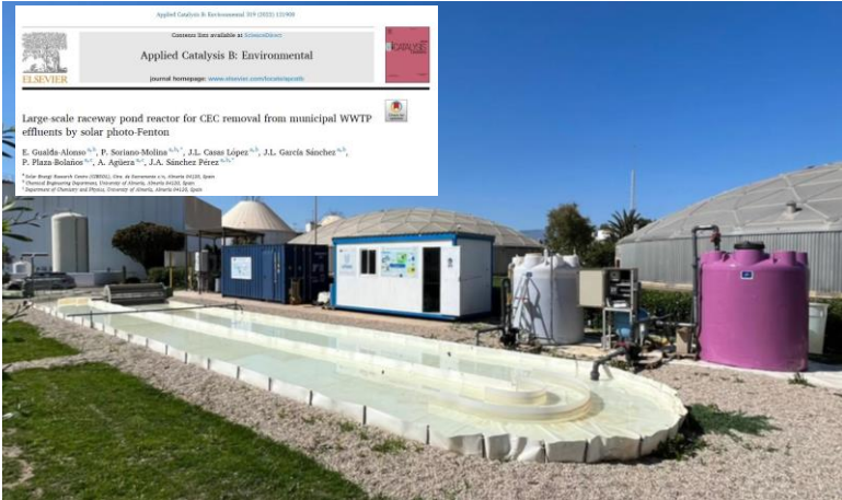
Demo plant 100 m 2 (18 m 3 )
